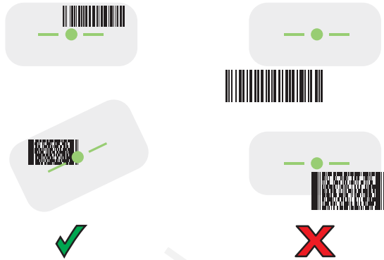
Figure 18 RS6100 Aiming Pattern
