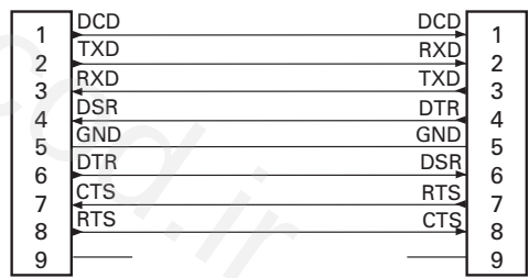
DB-9S Connector to DCE Device
