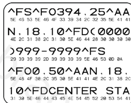
Figure 22 • Communications Diagnostics Test Label
