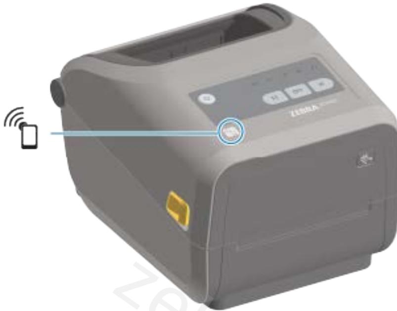
Figure 1 Print Touch Location (Passive NFC)
